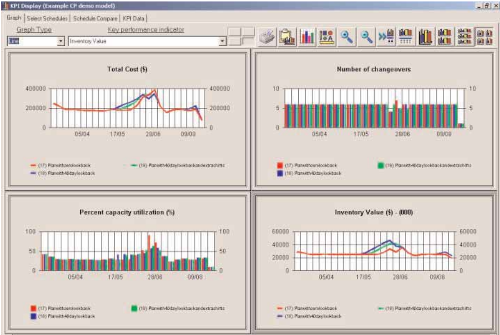
Figure 3: Key Performance Indicators illustrate the tradeoff between plant utilisation, production cost, changeover frequency and inventory value
